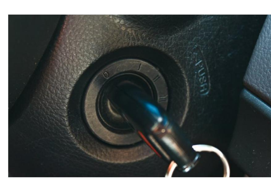
Turn the key to the "Off" position within 45 seconds of finishing step 2, and then turn it back to the "On" position for another 10 minutes and 30 seconds.
